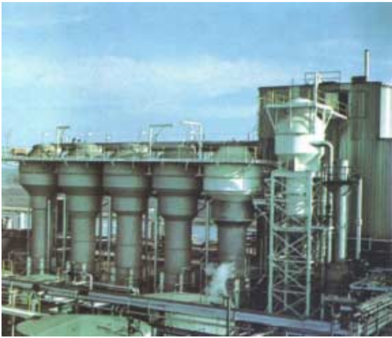
At left: Five effect LTV rising film evaporator with falling film concentrator, concentrating hydrolysate liquor.
