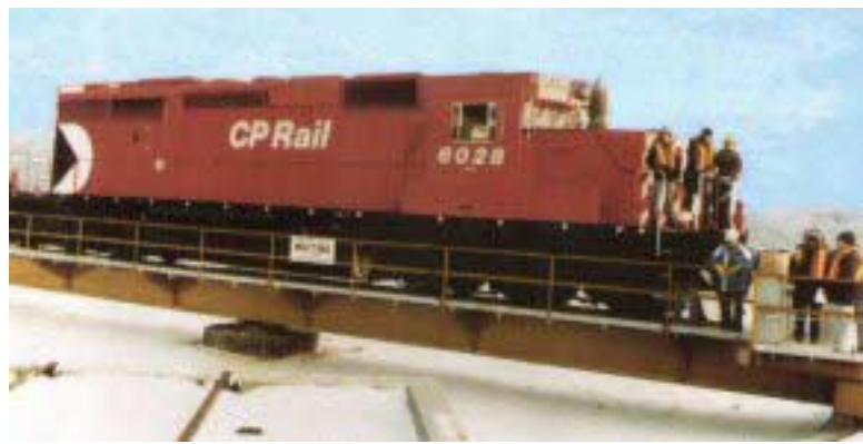
Top Photo – Whiting "Robot" progression system automatically moves cars through work stations in repair shop.
