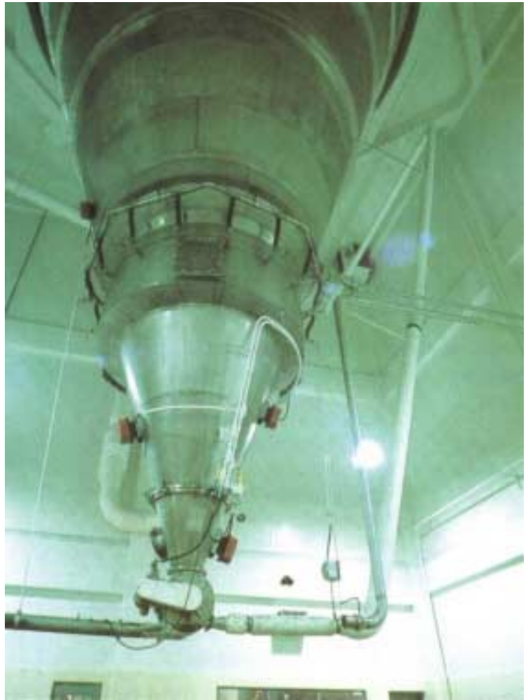
Right: Lower portion of a 110 ft. high Swenson parallel flow spray dryer.
