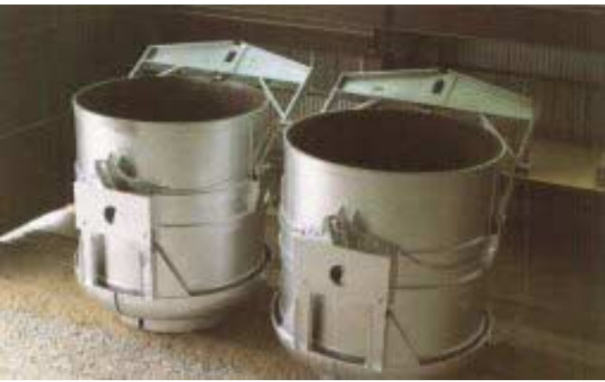
Left – 1200 cu.ft. capacity electric arc charging furnace buckets used in specialty steel making operations.
