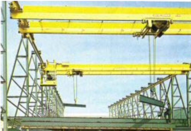
Above – Whiting 30/10 ton, centre mounted cab crane in melt shop of major farm equipment manufacturer.
