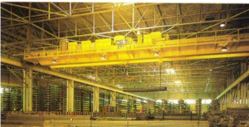
Below – Cab-operated 25 ton capacity industrial crane, custom designed by Whiting to efficiently handle long loads.
