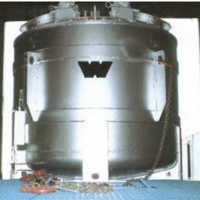
Left – Molten metal Handling vessel for special, non-ferrous applications.
