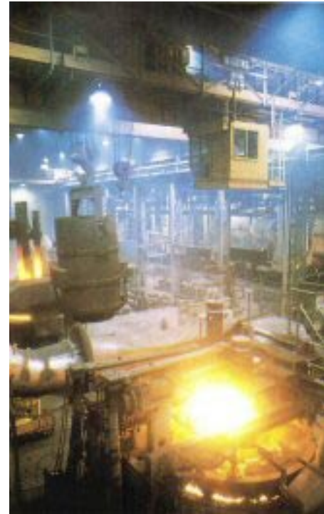
Above – Whiting 30/10 ton, centre mounted cab crane in melt shop of major farm equipment manufacturer.
