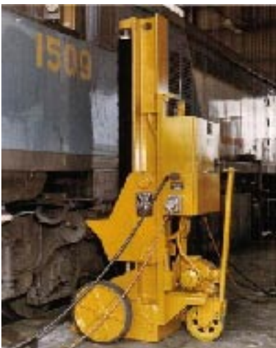
Below – A Whiting portable electric jack that can meet the requirements of dozens of unique lifting operations. Jack capacities range from 15 to 60 tons.
