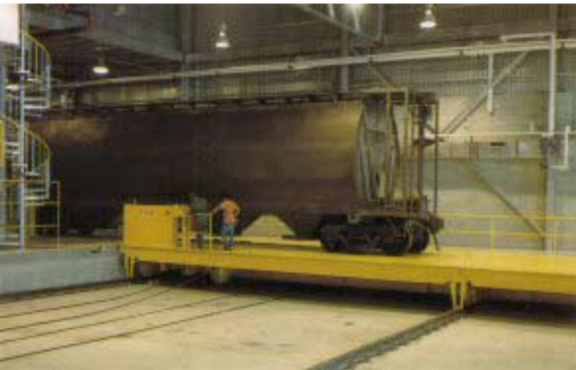
Above – Covered hopper car being positioned on Whiting Transfer Table for transfer to one of four paint system tracks.
