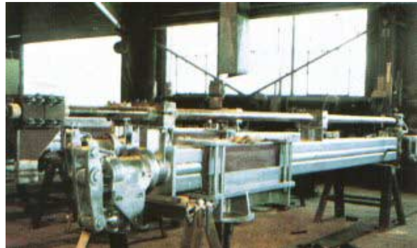
Below – Furnace components after disassembly in Whiting plant ready for shipment to installation site.
