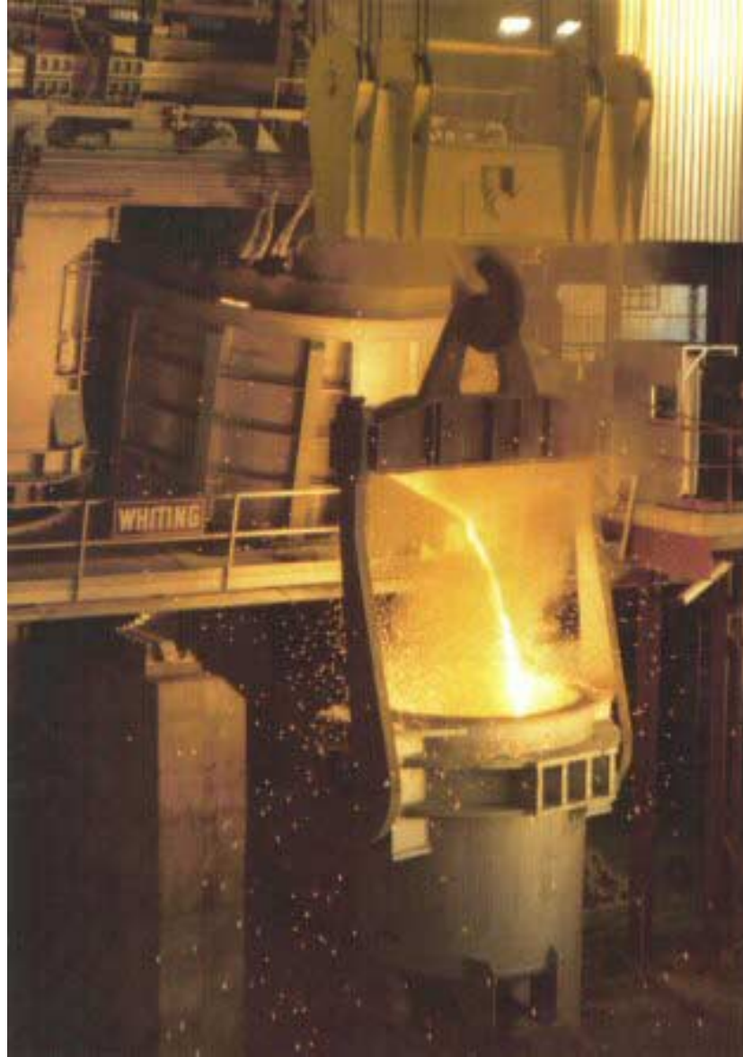
Above – 70 Ton Capacity Whiting-Volta Electric Arc Furnace shown during tapping in a specialty steel mill.
