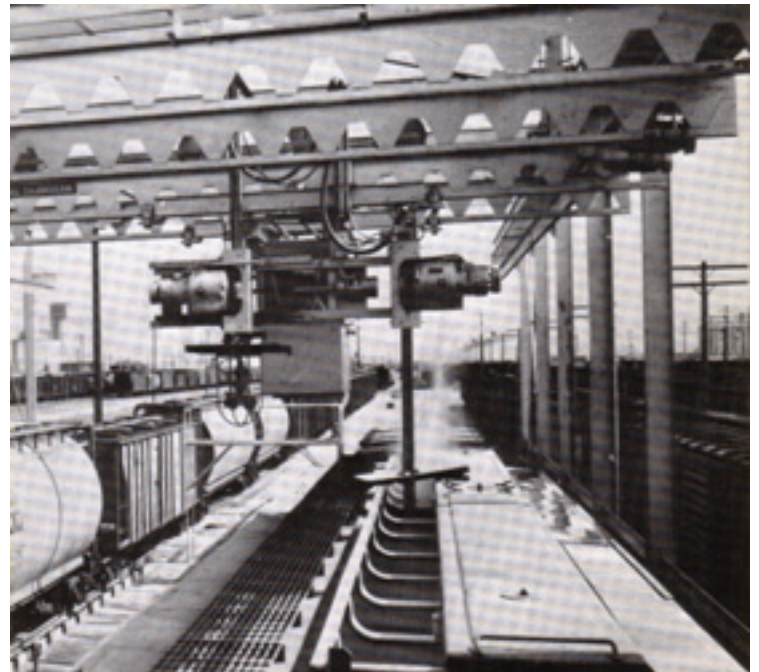
Only one wand is lowered for cars with single row of openings.
