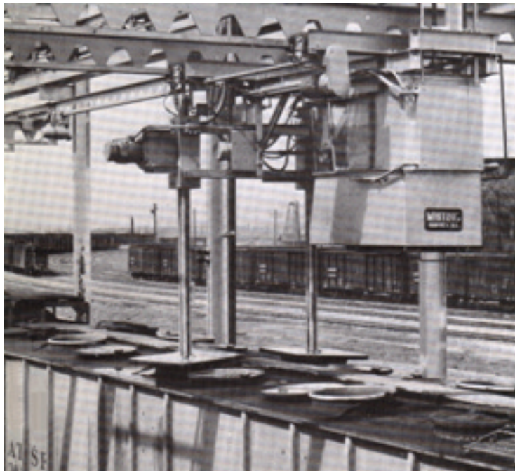
Close-up shows application of dual wand in car with double row of top openings.
