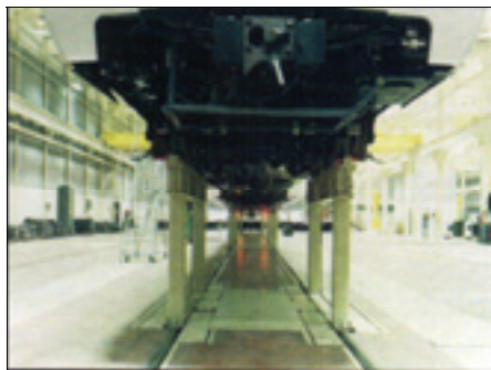
Construction is arranged so that the entire underside of the car is free of obstruction.
