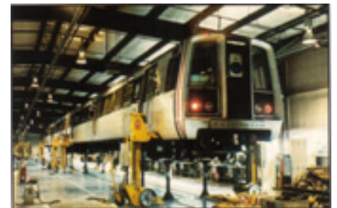
Standard portable electric jacks with special lifting brackets for metro car hoisting.
