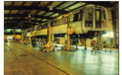
Standard portable electric jacks with special lifting brackets for metro car hoisting.
