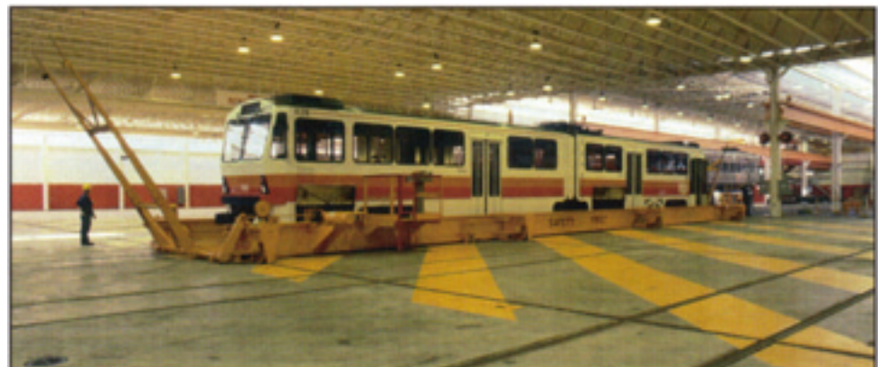
Pitless transfer table transporting articulated pair of metro cars.
