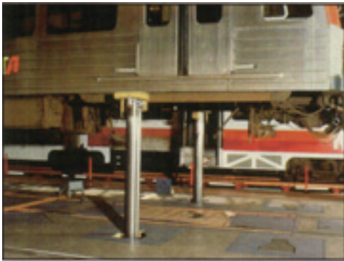
Body stands support the car(s) in a level position during truck removal.
