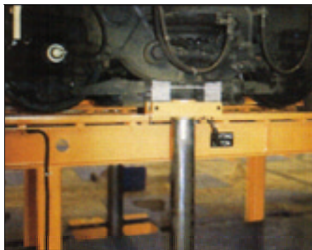
Wheel spinning posts raised and locked into position. When not in use the spinning posts are stored in recesses adjacent to the rails.
