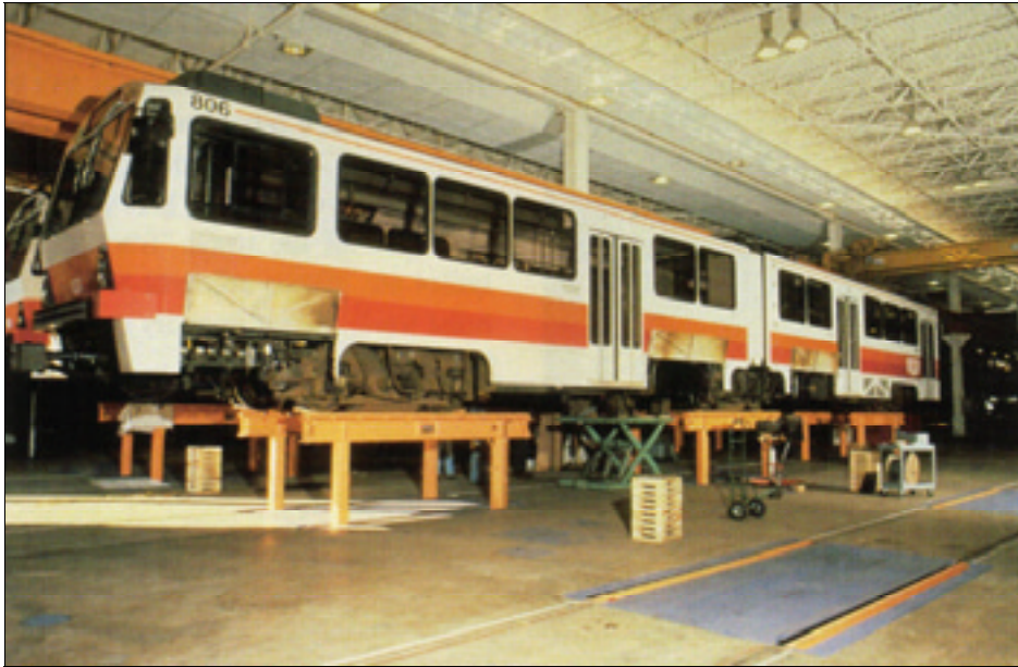
Car hoists raise pair of metro cars to a convenient height for worker access to underbody components.
