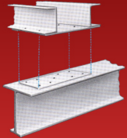
Close tolerance key plates are accurately aligned by an optical instrument and welded to the bridge girder of a single girder crane. The key plates fit into key slots machined in the end truck load bars and provide rigid and square connections of the girder to the trucks.
