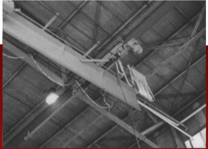
Single girder 4-wheel end truck driven by a No. 24-9 tractor drive.
