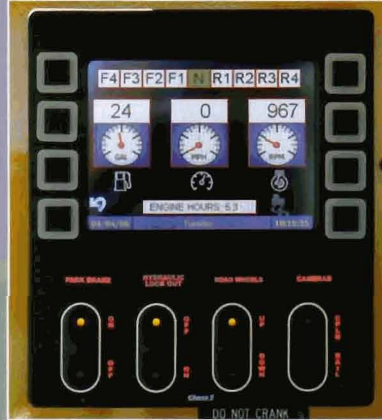
Command Master Control System
