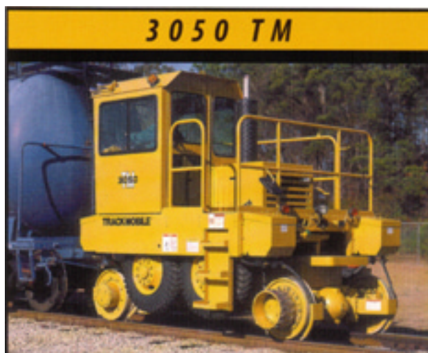
32,620 lbs. [14,796 kg] Double Coupled, 21,230 lbs. [9,630 kg] Single Coupled Tractive Effort • 29,850 lbs. [13,540 kg] Vehicle Weight • 4 cylinder Turbo-charged Diesel Engine • Three Speed Cable Controlled forward & reverse Transmission • One heavy duty, cast steel Weight Transfer Couplers • Fold-away Steps for transport purposes.
