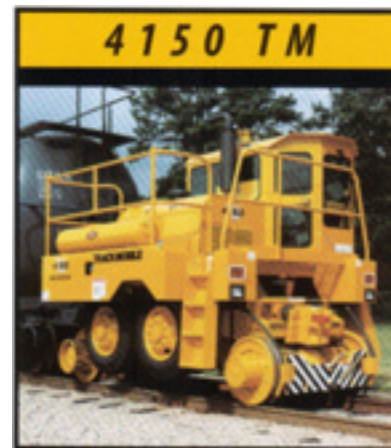
42,135 lbs. [19,112 kg] Double Coupled, 26,460 lbs. [12,002 kg] Single Coupled Tractive Effort • 32,680 lbs. [14,873 kg] Vehicle Weight • 6 cylinder Turbo-charged Diesel Engine • Four Speed Electronically Controlled forward & reverse Transmission • Two heavy duty, cast steel Weight Transfer Couplers • Dual controls for rail operation
