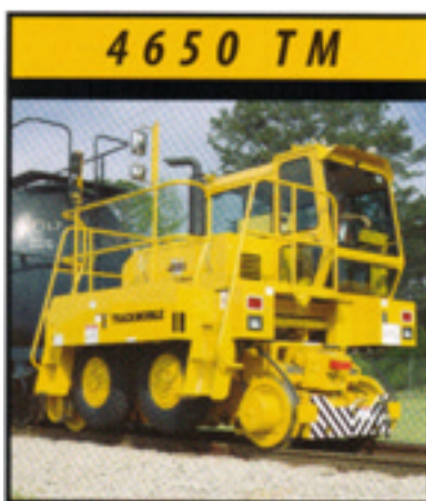
46,500 lbs. [21,092 kg] Double Coupled, 31,500 lbs. [14,288 kg] Single Coupled Tractive Effort • 47,000 lbs. [21,319 kg] Vehicle Weight • 6 cylinder Turbo-charged Diesel Engine • Four Speed Electronically Controlled forward & reverse Transmission • Two heavy duty, cast steel Weight Transfer Couplers • Dual controls for rail operation
