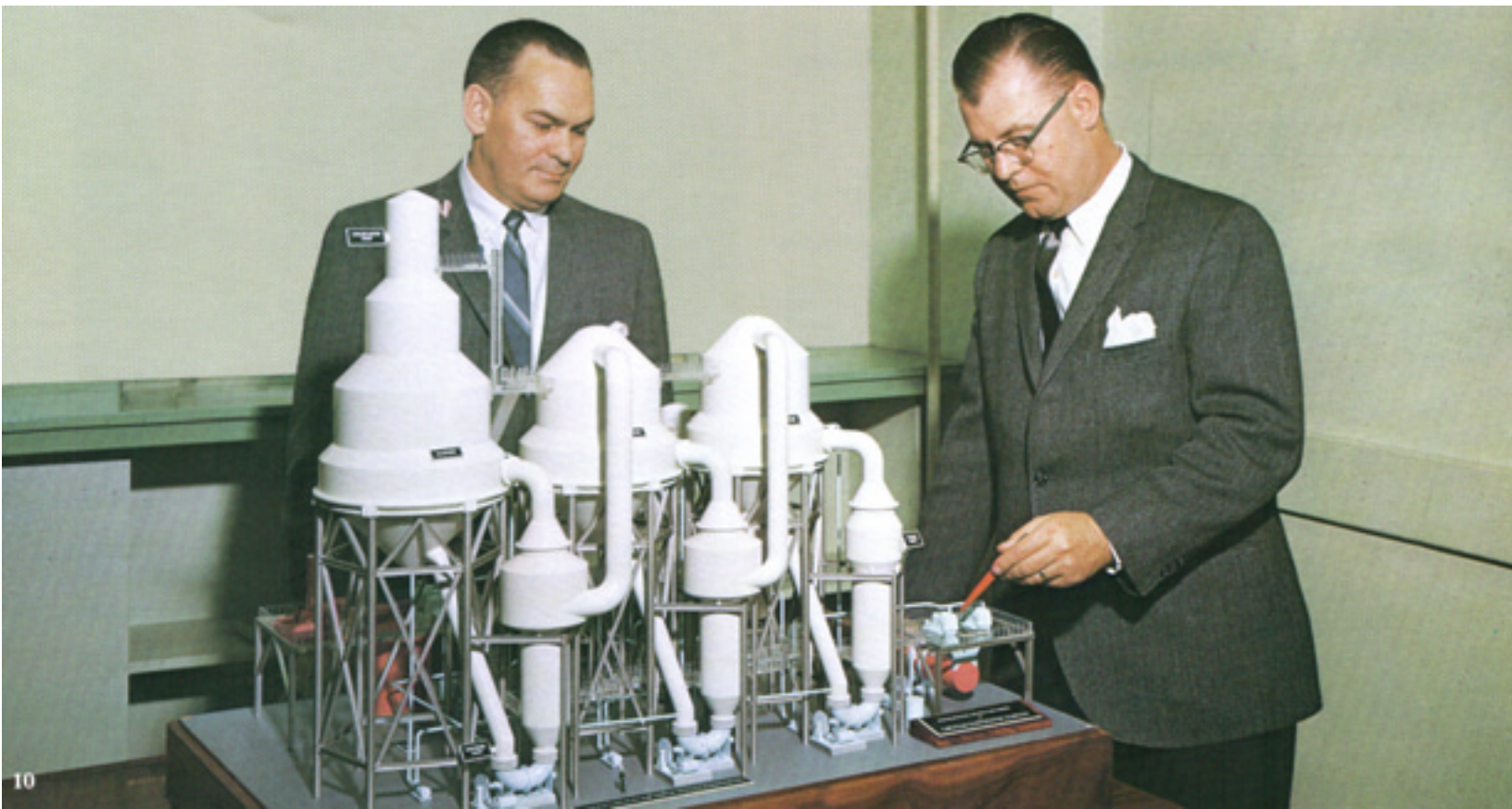
SWENSON two-stage forced-circulation evaporative crystallizer at Armour Agricultural Chemical Company
