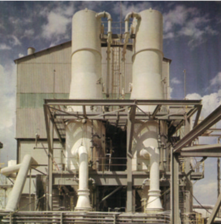
SWENSON two-stage forced-circulation evaporative crystallizer at Armour Agricultural Chemical Company
