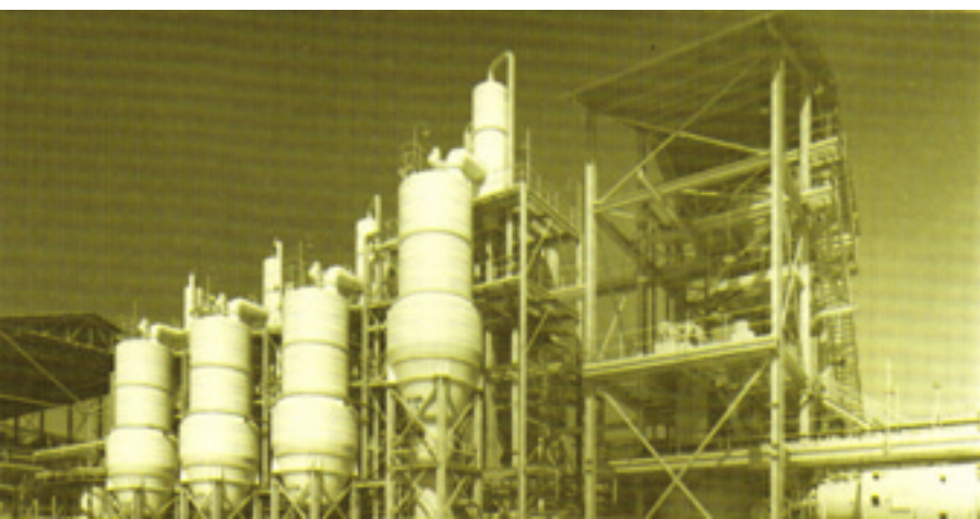
Eight SWENSON DTB units produce potassium chloride from Dead Sea brine at a rate of 58 tons per hour
