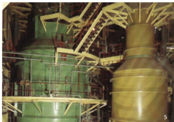
Two DTB Crystallizers used for the production of potash at Cleveland Potash, England
