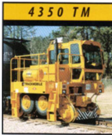
43,520 lbs. [19,740 kg] Double Coupled, 27,840 lbs. [12,628 kg] Single Coupled Tractive Effort • 36,870 lbs. [16,723 kg] Vehicle Weight • 6 cylinder Turbo-charged Diesel Engine • Four Speed Electronically Controlled forward & reverse Transmission • Two heavy duty, cast steel Weight Transfer Couplers • Dual controls for rail operation
