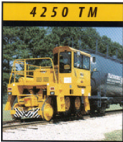
42,814 lbs. [19,420 kg] Double Coupled, 27,139 lbs. [12,310 kg] Single Coupled Tractive Effort • 34,740 lbs. [15,758 kg] Vehicle Weight • 6 cylinder Turbo-charged Diesel Engine • Four Speed Electronically Controlled forward & reverse Transmission • Two heavy duty, cast steel Weight Transfer Couplers • Dual controls for rail operation
