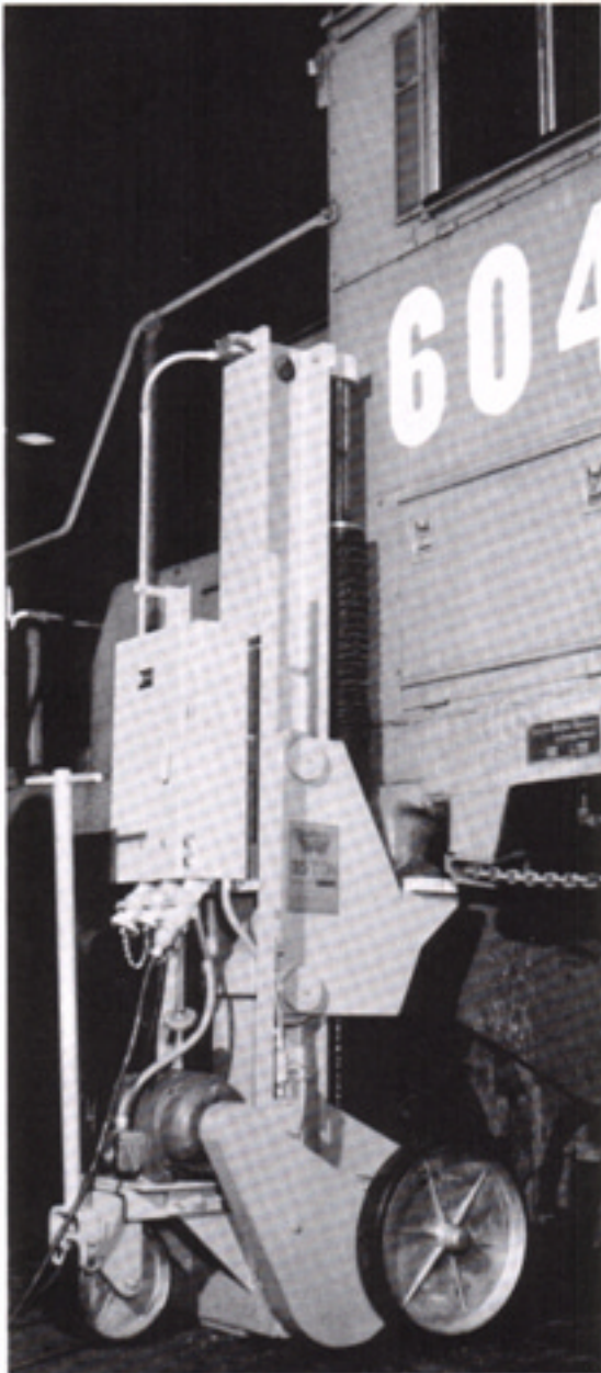
Jack models MA, MAE, MB and MC are similar in appearance but vary in low bracket height (2'3"-2'9") and effective lift (55"-67"). Jack adaptors are available in several sizes to fit your requirements.
