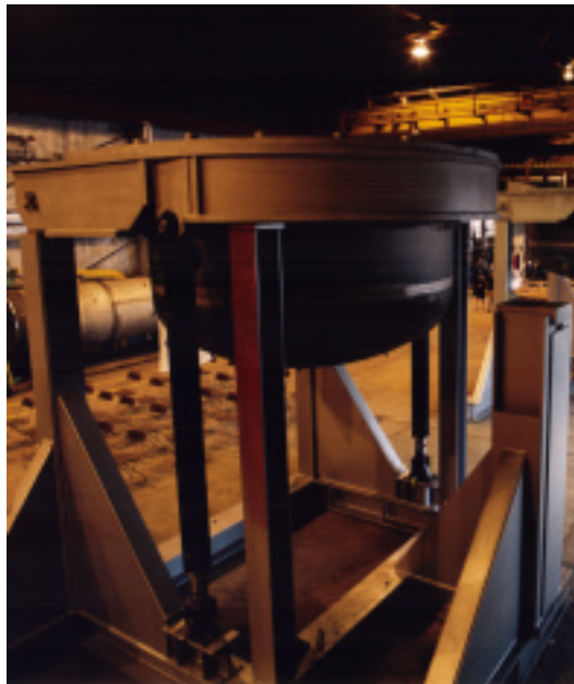
Removable shell mineral fusion furnace base assembly – Rear View
