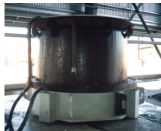
Special processing applications equipment - water cooled "Higgins" type furnace shell for fused oxides
