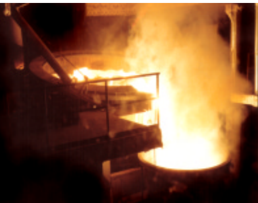
Tilt pouring of molten mineral oxides into a water-cooled mold
