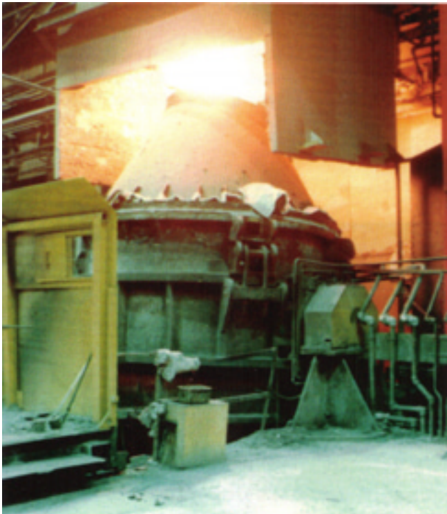
50 ton capacity AOD unit capacity blowing a heat of high quality stainless steel mill products
