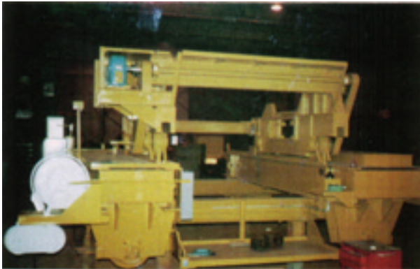
85 ton capacity, bottom tapping ladle ingot pouring transfer car with traversing carriage arrangement
