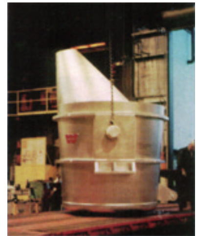
Ferro-alloy application lip pouring crane ladle with detachable bail feature
