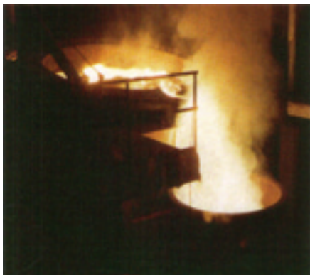
Tilt pouring of molten mineral oxides into a water-cooled mold
