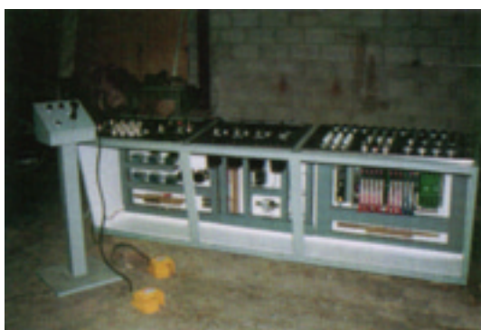
Custom-built, electric arc furnace operator's control console complete with integrated PLC, tilt control pedestal and dead man's switch. Mineral fusion operation
