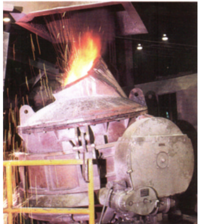
Operating view of AOD used in the production of small stainless steel castings – foundry application
