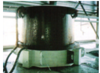
Special processing applications equipment - water cooled "Higgins" type furnace shell for fused oxides
