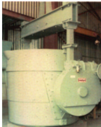
35 ton, motorized, lip pour crane ladle, with non-detachable bail for iron and steel
