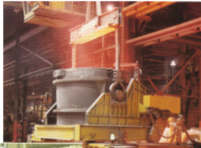
Whiting 50-ton capacity ingot pouring car with DC drive and hydraulic braking. Accurately positions ladle at one or more rows of ingot molds.
