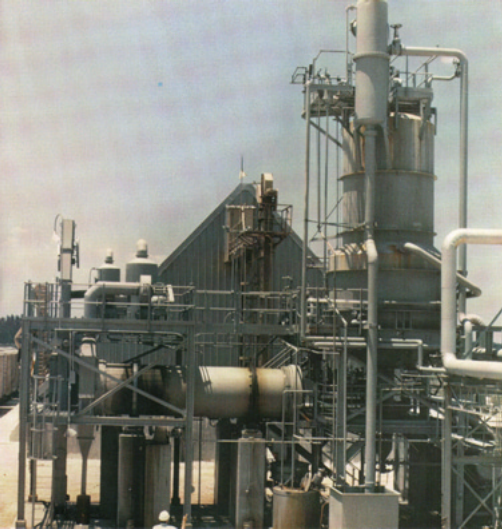
SWENSON DTB crystallizer with SWENSON rotary dryer.
