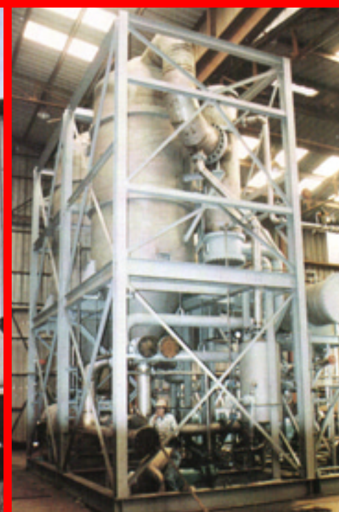
SWENSON skid mounted forced circulation crystallizer.
