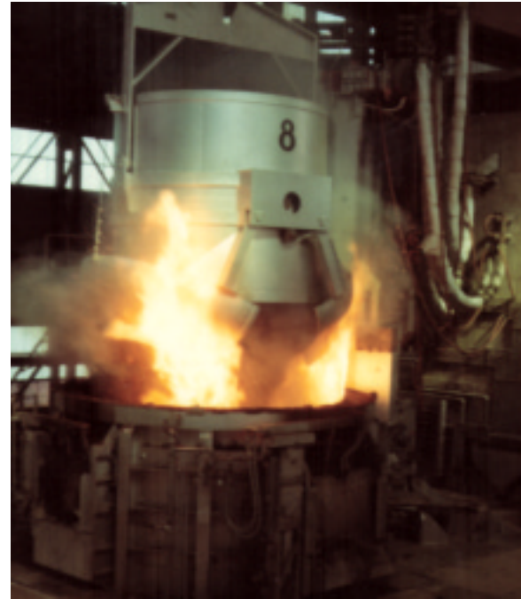
1500 cubic foot capacity, electric arc furnace charging bucket - scrap steel melting application
